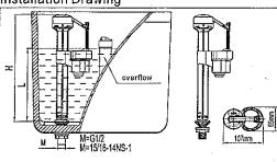
The height of "H" & "L" doesn't include the height of triangle seal. 10" fill valve pipe H=254mm L adjustable range 133-185mm 11" fill valve pipe H=287mm L adjustable range 166-218mm
