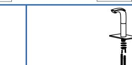
2. Screw and hand tighten the hot and cold flexible hoses to the faucet. DO NOT use a wrench to tighten hoses, as this may damage the hose and/or hose threads
