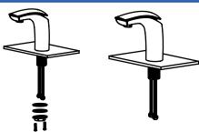
4. Reinstall the rubber washer, followed by the metal washer and lock nut. Hand tighten, then tighten further using a screw driver to tighten the lock nut.
