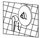
Put on the handle, then tighten the screw.
