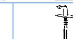
2. Screw and hand tighten the hot and cold flexible hoses to the faucet. DO NOT use a wrench to tighten hoses, as this may damage the hose and/or hose threads
