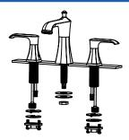
1. Remove three way connector. Remove mounting hardware assembly.
