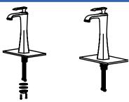
4. Reinstall the rubber washer, followed by the metal washer and lock nut. Hand tighten, then tighten further using a screw driver to tighten the lock nut.
