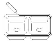
**7.** Position and align sink over the countertop opening and press sink
