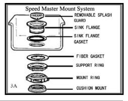
When the cushion mount is installed correctly, the lip of the sink flange fits into the groove on the inside of the cushion mount and mount ring can be pulled downward over cushion mount and will be free to rotate. The bottom bead of the cushion mount acts as a gasket between the bottom of the sink flange and the top of the disposer. See illustration 3G.
