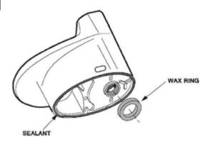
Turn toilet bowl down onto a towel or cushioned surface, Place the wax ring around the draining outlet of the bowl, and press firmly. Apply a thin bead of sealant around toilet base.
