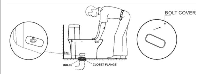
A. Position toilet squarely to wall, and with a rocking motion, press bowl down fully onto wax ring and flange. Next, tighten nuts until toilet is firmly seated on floor.
