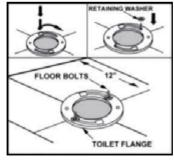
Insert floor or bolts into flange channel with bolt head down. Use plastic retaining washers to hold the bolts in place, Floor bolts should be parallel to wall and 6"( 152mm)apart.
