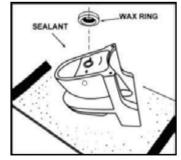
Turn toilet bowl down onto a towel or cushioned surface. Place the wax ring around the draining outlet of the bowl, and press firmly. Apply a thin bead of sealant around toilet base.
