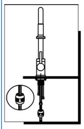
2. Proper installation of the hose weight kit will ensure that the spray head retracts smoothly. On the spray side of the hose, measure 15" down from the body of the faucet and install the hose weight kit here. Pull out on the spray head. It should move easily and retract smoothly. Reposition the hose weight kit as necessary. Make sure that the hot and cold supply hoses do not interfere with the spray hose. they can be repositioned slightly if necessary.
