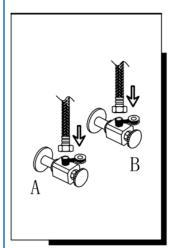
4. Attach the two flexible hoses to water supply.
