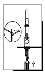
3. Screw and tighten the flexible hoses to the faucet. Do not allow the water supply brass tube to twist.
