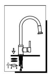
1. Install faucet through center hole, assembly washer & metal washer onto faucet. Tighten with lock nut.
