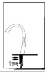
1. Insert faucet through center hole, assembly washer & metal washer, onto faucet and tighten with lock nut.
