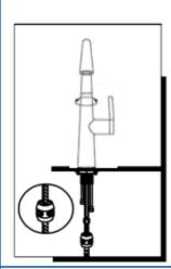
2. Proper installation of the hose weight kit will ensure that the spray handle retracts smoothly.
