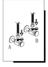
Attach two flexible hoses to water supply.
