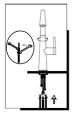
3. Screw and tighten the flexible hoses to the faucet. Do not allow the water supply brass tube to twist.
