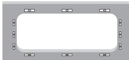
**5.** Loosely attach mounting brackets to the countertop, parallel to the cutout opening using proper fasteners.
